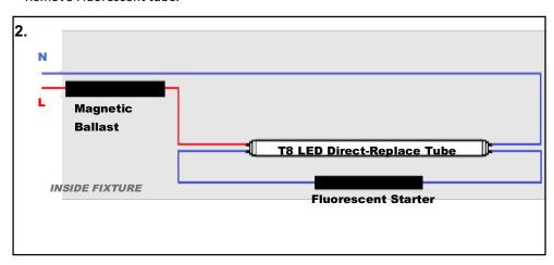
**STEP 2:** Install T8 LED Direct-Replace Tube.
