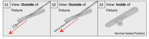
Step 1 (S1). Align the paddle with the cable to allow the cable bead, cable length, and paddle to pass through a Ø6.4mm hole.
