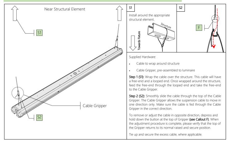
Part of the suspension kit is assembled into the light fixture. However, if for some reason the suspension kit is not completely assembled into the fixture, follow the following procedure to reattach the cable into the luminaire.
