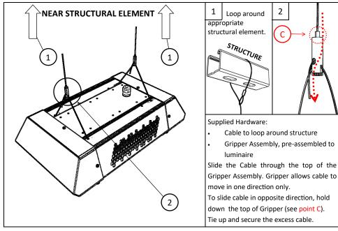
Part of the suspension kit is assembled into the luminaire. However, if for some reason the suspension kit not completely assembled into the fixture. Follow the following procedure to reattach the cable into the luminaire.
