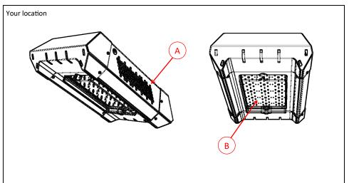
Holes (see point A) on the side of the housing allow for ventilation of heat from the housing. Do not mount fixture where this ventilation may be obstructed.
