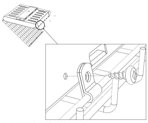
Mesh guard covers entire illuminating face of the fixture. Total of 6 screws secure the mesh guard to the fixture housing.
