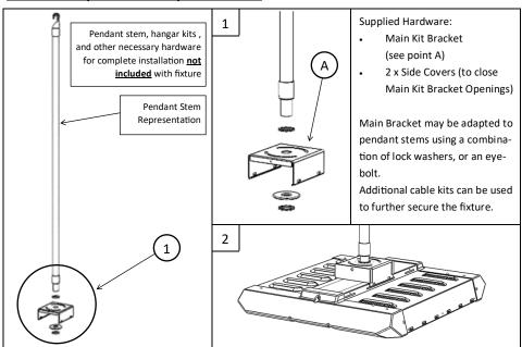
The Main Bracket should hook into the slot on both sides at the center of the fixture (see point B). Align and secure the bracket to the fixture with the four provided fasteners (see point C) at both sides of the bracket.
