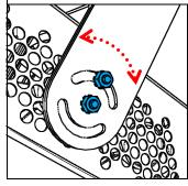
Adjust the orientation of the fixture. Re-tighten depicted bolts on both sides of the fixture. Bolts depicted in in the image on left are supplied with fixture.
