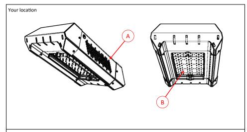
Holes (see point A) on the side of the housing allow for ventilation of heat from the housing. Do not mount fixture where this ventilation may be obstructed.
