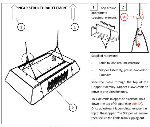
Part of the suspension kit is assembled into the luminaire. However, if for some reason the suspension kit not completely assembled into the fixture. Follow the following procedure to reattach the cable into the luminaire.
